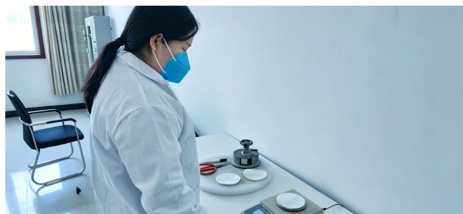
INSTRUMENT 03 · GRAMMAGE CHECK Weight / thickness gauge · 克重检测
